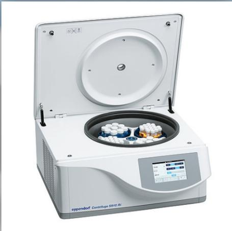
A high-speed centrifuge is used to separate substances of different densities in a liquid medium that operates on the principle of centrifugal force. The facility has a total of seven refrigerated centrifuges and two minispins. All the centrifuges are of Eppendorf make and their speed varies from 10-15000 rpm.
